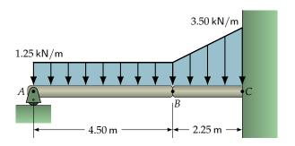
There is a roller at A, a pinned connection at B and a fixed connection at C. Determine the reactions at A and C.
