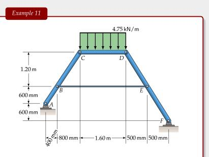
Determine the reactions at A and F, and the tension in cable BE.
