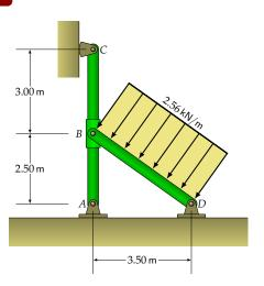
There is a smooth collar at B, a rocker at C and pinned connections at A and D. Determine the force that the collar at B exerts on member BD, and the reactions at A and D.
