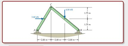
The pinned connections at A and B each have two unknown reaction components so we cannot do anything 'globally' with the whole frame. Separate the two frame members and draw the free-body diagrams.
