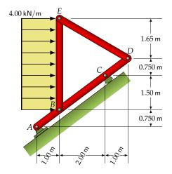
Determine the reactions at A and C, and the internal force in two-force member DE.
