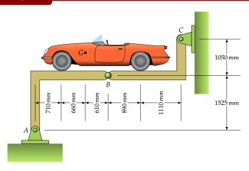
The sports car has a mass of  $1100 \, \mathrm{kg}$  and centre of gravity at G. Half of the mass is supported by the frame shown (a similar frame, hidden from view, supports the other half). All connections are pinned. Determine the reactions at A and C.
