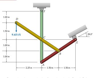
Determine the magnitude of reactions in A, B and C due to the  $9.65\,\mathrm{kN}$  load.
