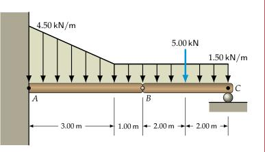
There is a fixed connection at A, a pinned connection at B and a roller at C. Determine the reactions at A and C.
