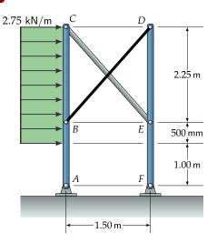
Find the forces in cable BD and strut CE, and the reactions at A and F.
