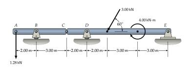
There are frictionless rollers at B and D and a pinned connection at E. Determine the reactions at B, D and E.
