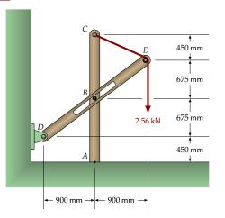
There are smooth pegs B and E, and a pinned connection at D. A is fixed connection. Determine the reactions at A and D.
