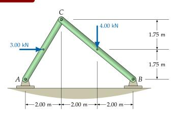
Determine the components of the reactions at A, B and C.
